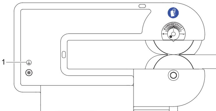
Fig. 3 Earthing Connection
